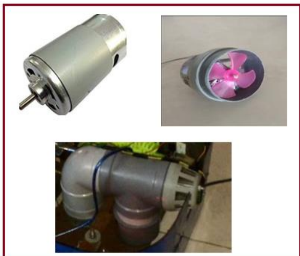
Figure 4: High speed DC motor, blower fan and dust collector mechanism
