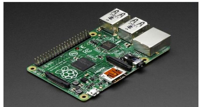
CPU, 512RAM.(Pi 1) Model B+, it also has: 2 USB ports, 26 GPIO pins, Full HDMI ports, Ethernet port, Combined
