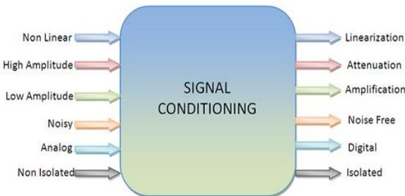
Signal conditioning is the manipulation of a signal that prepares it for the next stage of processing. Manipulating an analog signal in such a way that it meets the requirements of the next stage for further processing. Most common use is analog-to-digital converters Applications involve environmental or structural measurement, such as temperature and vibration, from sensors.
