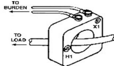
CT's are generally located in the main breaker panel or in branch distribution panels where space is always at a premium. CT's do not have to be installed 90 degrees to the conductor run they are generally held in place with plastic tie wraps. CT's with mounting feet are available if appearance is important and there is enough room to accommodate this type of mounting arrangement.
