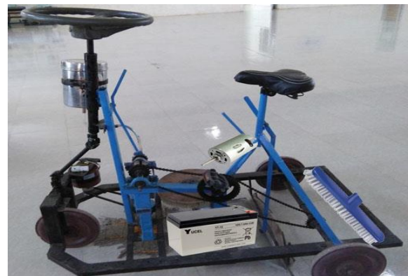
Figure 3.1: Modified Floor Cleaning Machine
