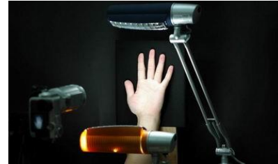
Figure 2 The palmprint and hand geometry image acquisition module (PHIA module).
