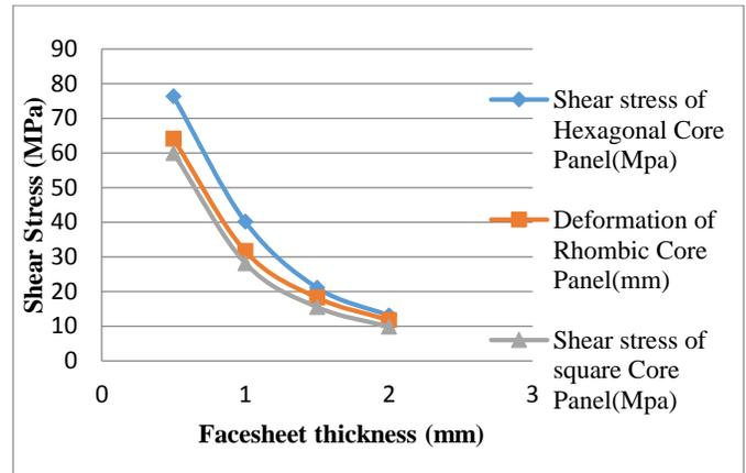
Fig.5.2: Shear stress of honeycomb panel with varying face sheet thickness
