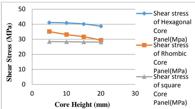
Fig.5.4: Shear stress of honeycomb panel with varying core height
