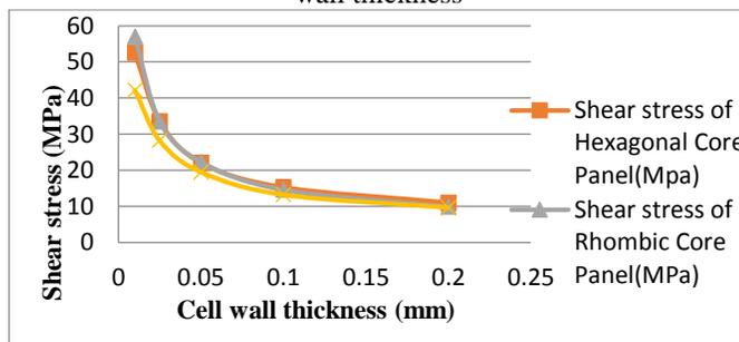
Fig.5.6: Shear stress of honeycomb panel with varying cell wall thickness
