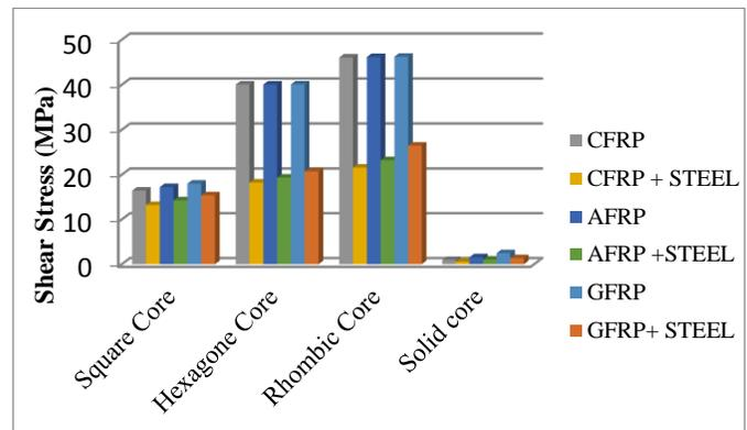
Fig.5.12: Comparison of Shear stress of panel with different cores (Moving load)
