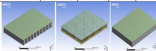
Fig.3.2: Model of honeycomb sandwich panels (Hexagonal, Square and Rhombic)
