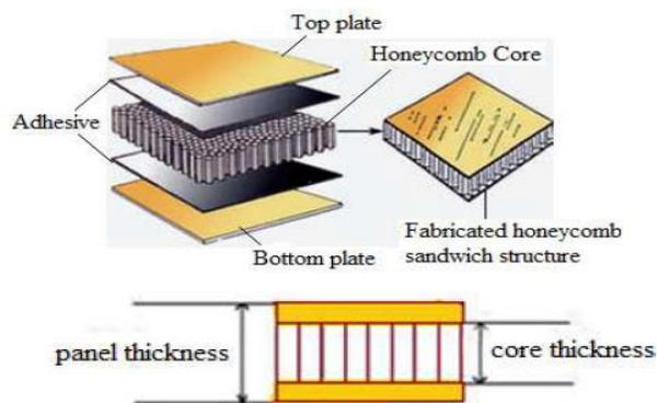
Fig.1.1: Honeycomb sandwich panel
