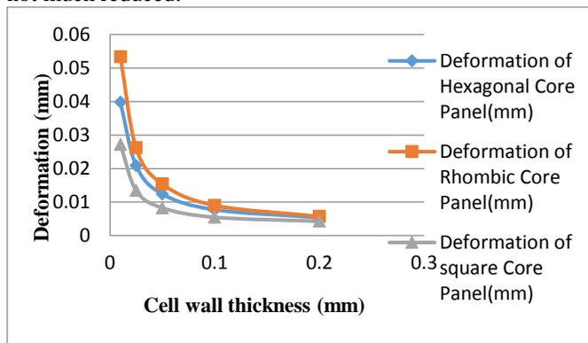
Fig.5.5: Deformation of honeycomb panel with varying cell wall thickness
