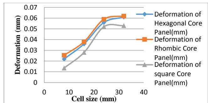
Fig.5.7: Deformation of honeycomb panel with varying cell size
