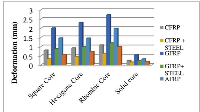
Fig.5.11: Comparison of deformation of panel with different cores (Moving load)
