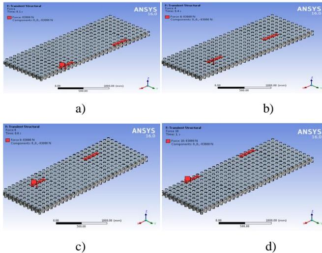
Fig.4.1: Moving load on deck panel at different time a) 0.1s b) 0.4s c) 0.8s d) 1s
