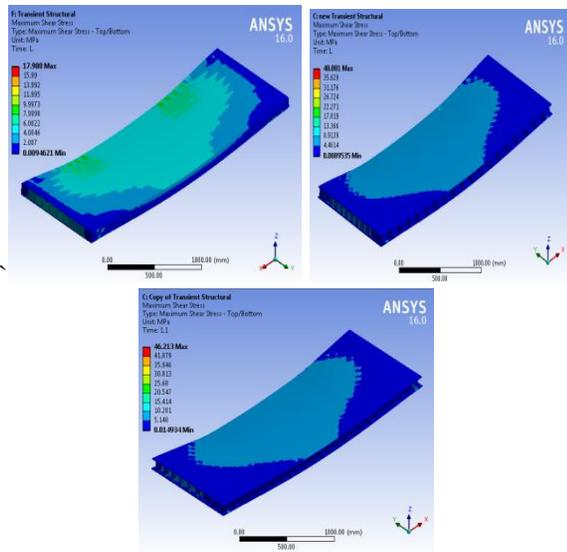
Fig.5.10: Shear stress of square, hexagon and rhombic core GFRP panel in transient analysis
