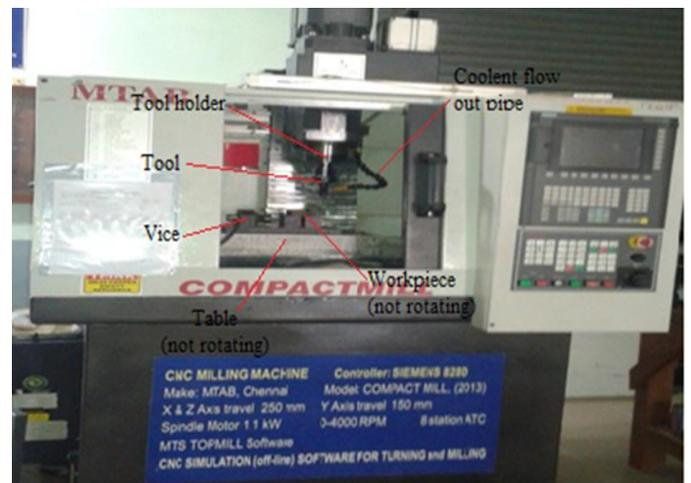
Figure no.01: Photographic view of experimental setup for machine
